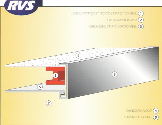
Fire Protection for Mezzanine Floor Edges. Replacement for Conventional Continuous Board Bulkhead. Pro-Case Fascia is a pre-formed, tailor made fire protection system for the protection of mezzanine floor edges against fire & is the perfect complement to our Pro-Case Column Casings. Pro-Case Fascia can afford up to 2 hours fire resistance. Tested WFRC
